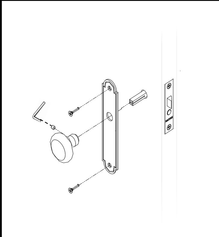
Secure knob & lever to spindle stem with Allen Wrench (provided)
